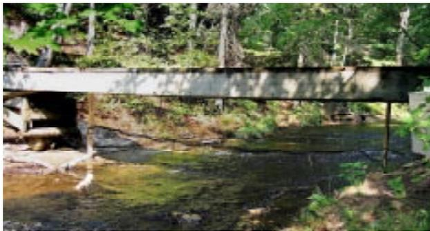
*Texas Instruments Radio Frequency ID station near the mouth of the Mosquito River, Pictured Rocks National Lakeshore. Reader, logger, and batteries are enclosed in a wooden box on the right (river left). The upper cable of the loop antenna is visible, suspended below the footbridge and above the stream; the lower cable is anchored on the stream bottom (John Wullschleger).*
