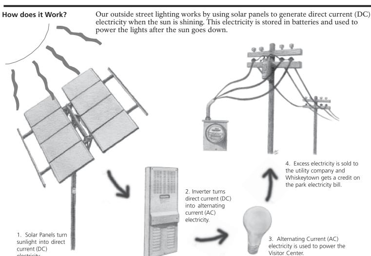
Whiskeytown's visitor center uses solar panels to run conventional plug -in electrical appliances by converting the direct current (DC) electricity produced by solar panels into alternating current (AC) electricity like what is delivered by the utility company by using a device called an inverter. When Whiskeytown generates more electricity than the visitor center is using, the excess energy is fed
