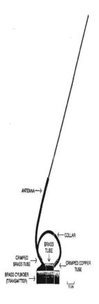
Figure. Radio transmitter design and attachment.
