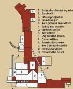
1924 Mill equipment is continuously added to and improved, and other additions are built to accommodate it. The Hancock jig addition built up the hill is expanded. Across the tracks, a Leaching Plant has been added to the Leaching Plant for wet Mill tailings, and both are in full swing.
