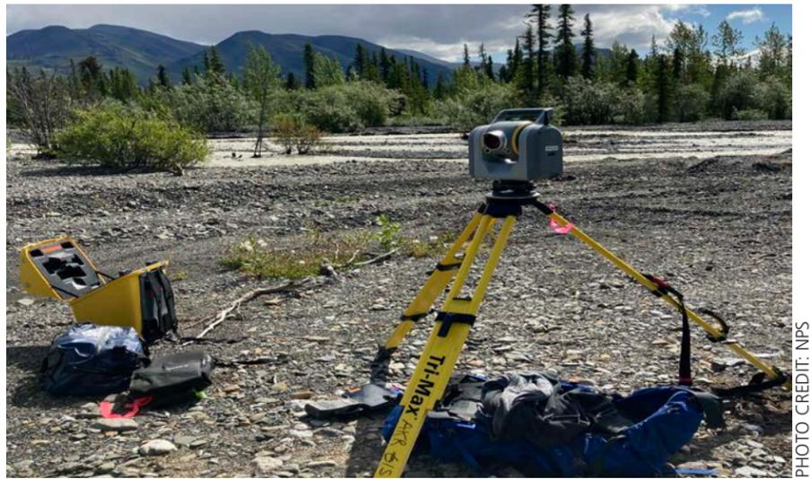
Pictured above is the SX10 terrestrial LiDAR Scanner used on Lost Creek in 2020.
