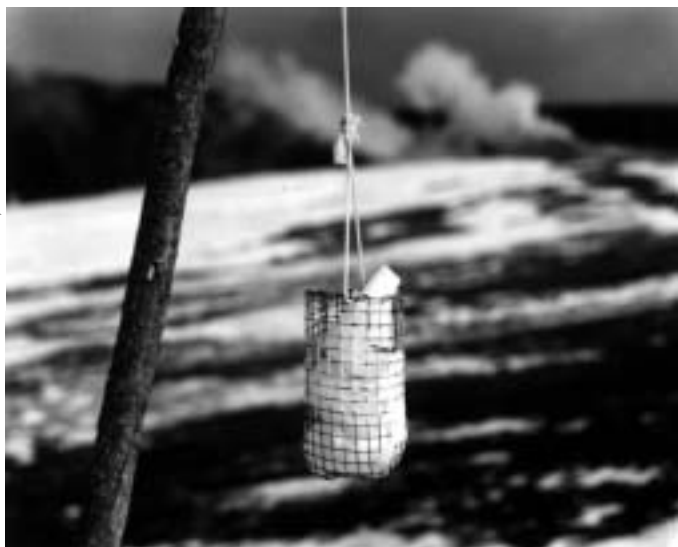
Basket of dry ice used for cloud seeding.
