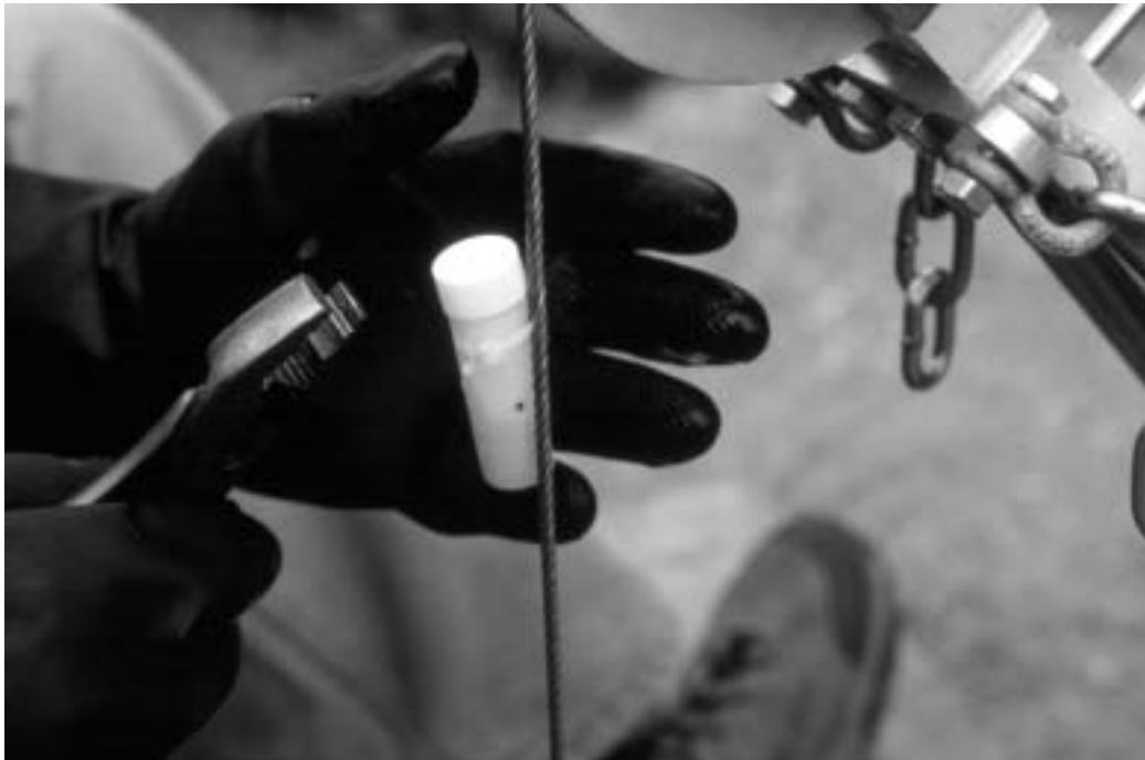
An in situ growth vial, designed to detect the presence of subsurface microbiota, is attached to a stainless steel cable for deployment into Yellowstone's Well Y-7.
