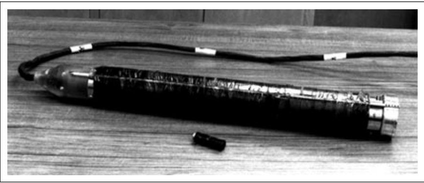
The video camera, in the foreground, is only about 2 inches in length. Behind it is the thermally-insulated container in which it is lowered into the conduit. The tape marks are at 1-foot intervals.
