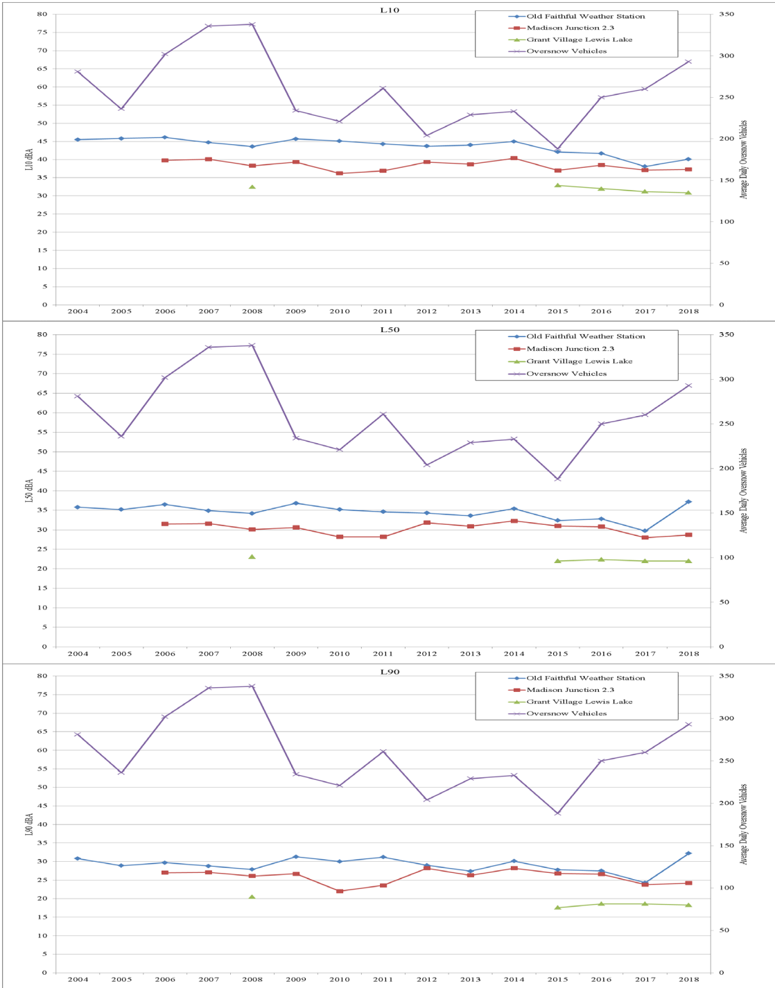
Figure 11. Long-term median L 10 , L 50 , and L 90 sound levels, 8 am to 4 pm, at two travel corridor and one developed area monitoring sites, and average daily number of oversnow vehicles of the winter use season by year, 2004-2018, YNP.
