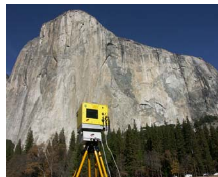
Figure 1. Ground-based laser scanner collecting digital topographic data for the southeast face of El Capitan, site of several large rock falls in 2010.
