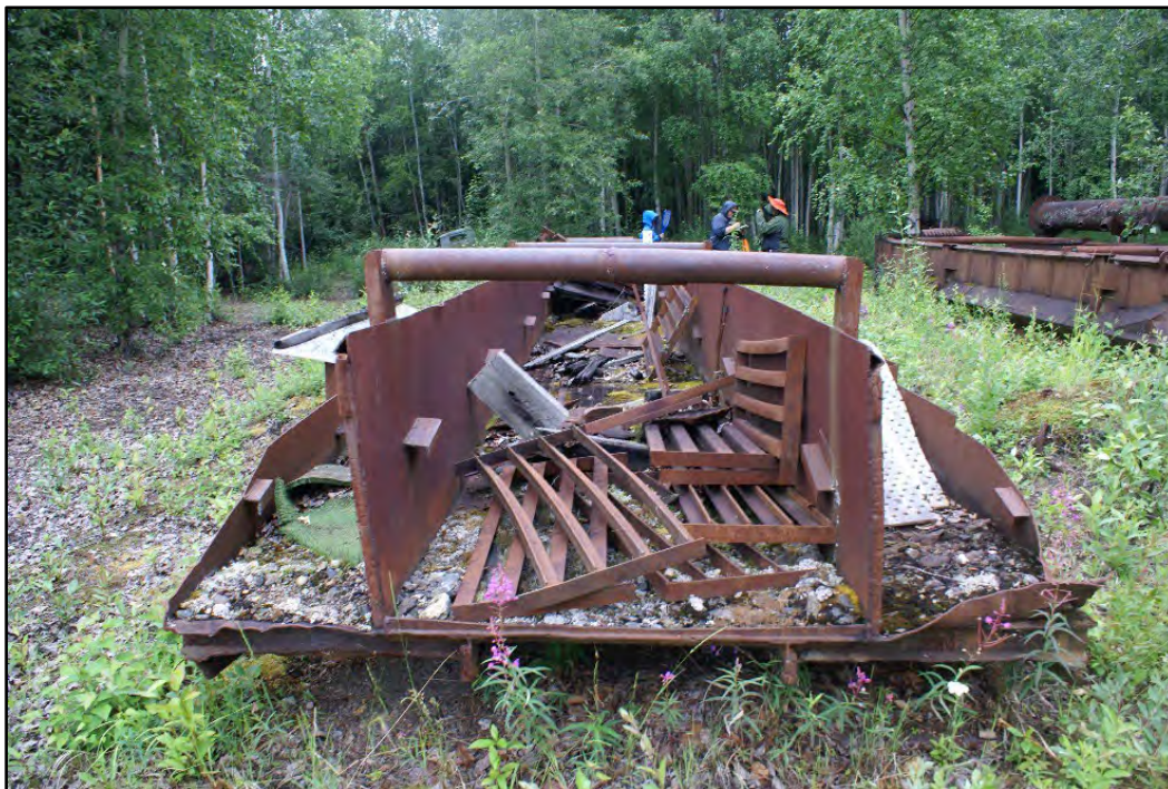
Photograph 6: Lower half of a sluice box used in the 1970s and 1980s
