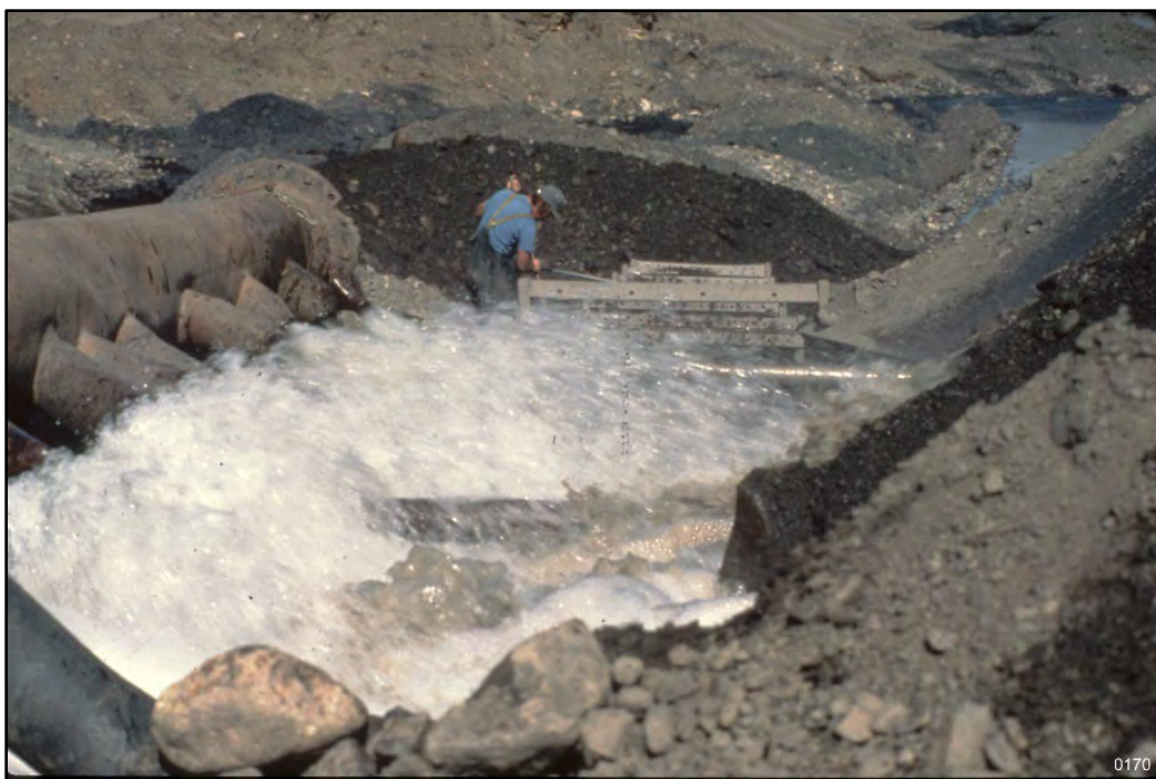
Figure 4: The "grizzly" section of the sluice box blasts incoming gravel, 1983
