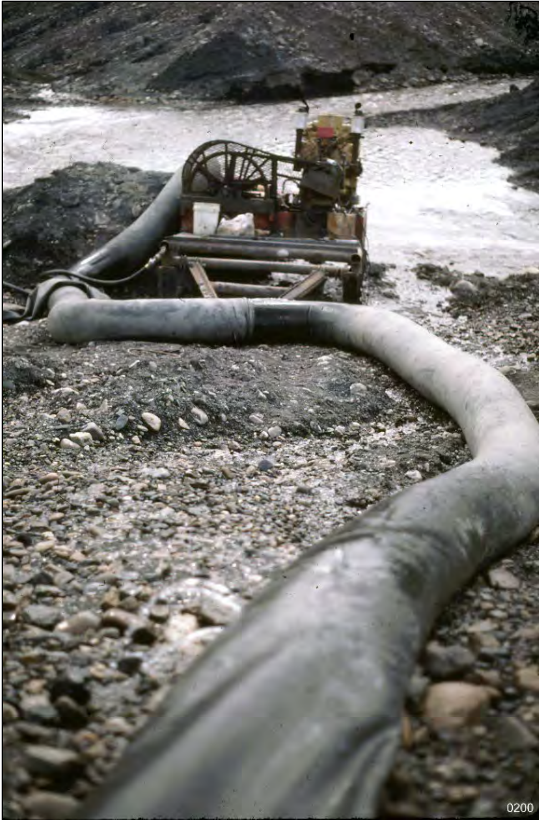
Figure 3: A pump supplies the sluice box's water jets for open-cut mining, 1983
