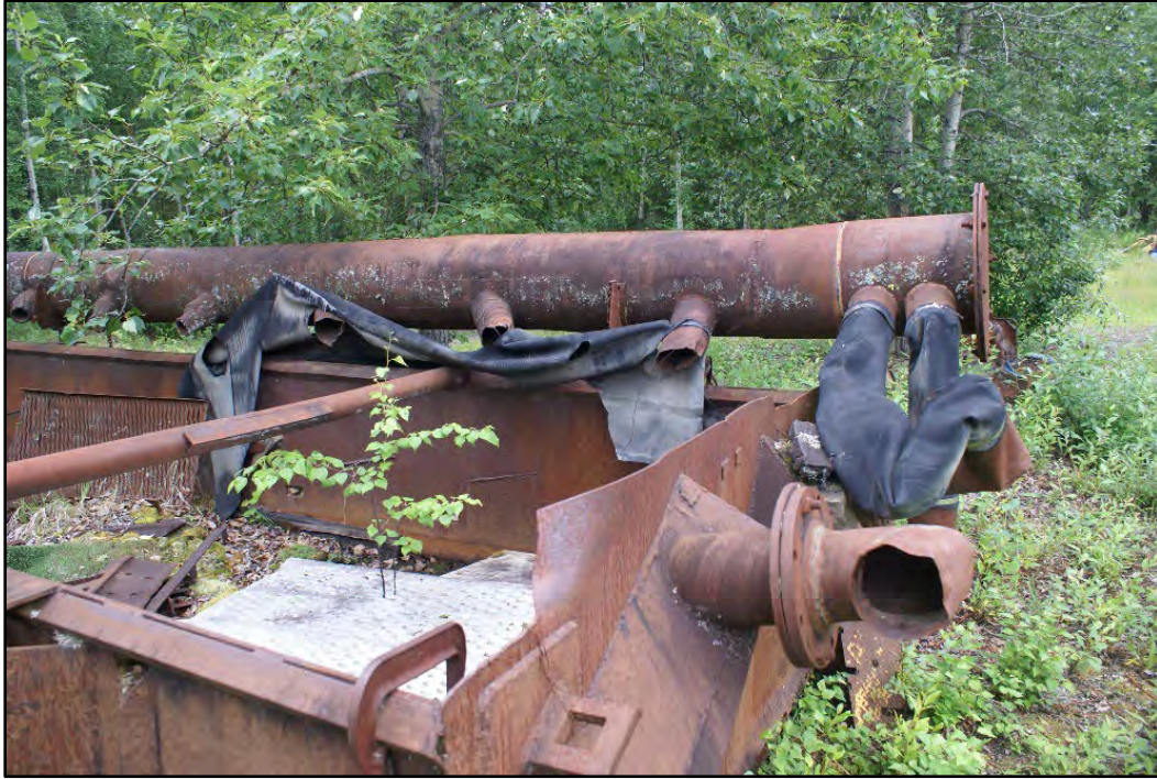
Photograph 7: Upper section of a sluice box with water jets and plastic mats
