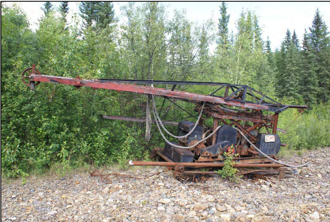
Photograph 4: Churn drill used 1930s to 1980s for measuring gold values at Coal Creek
