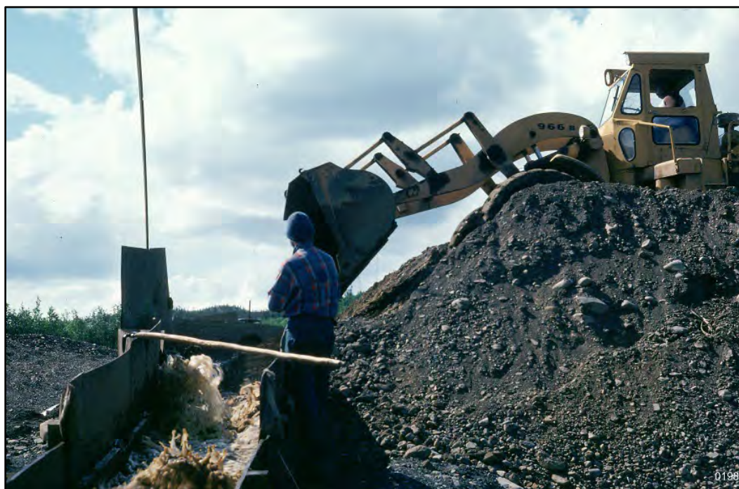
Figure 5: A front-end loader feeds gravel into the head of a sluice box, 1976
