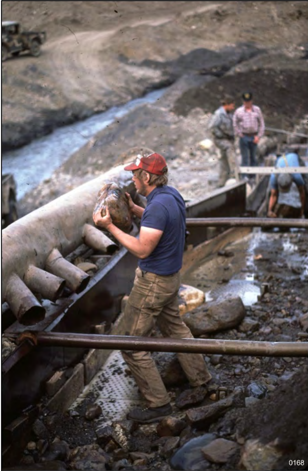
Figure 6: The "rock man" ejecting boulders from the grizzly section of the sluice box, 1983
