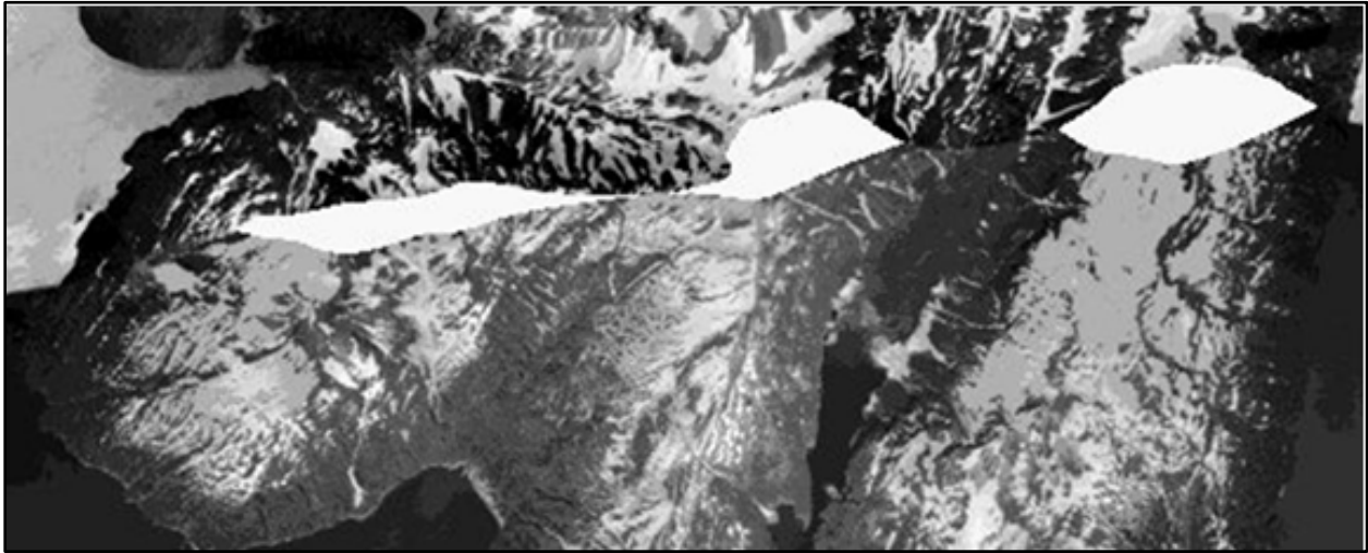
Figure 8. Missing data (shown in white) resulting from poor overlap between adjacent photographs.
