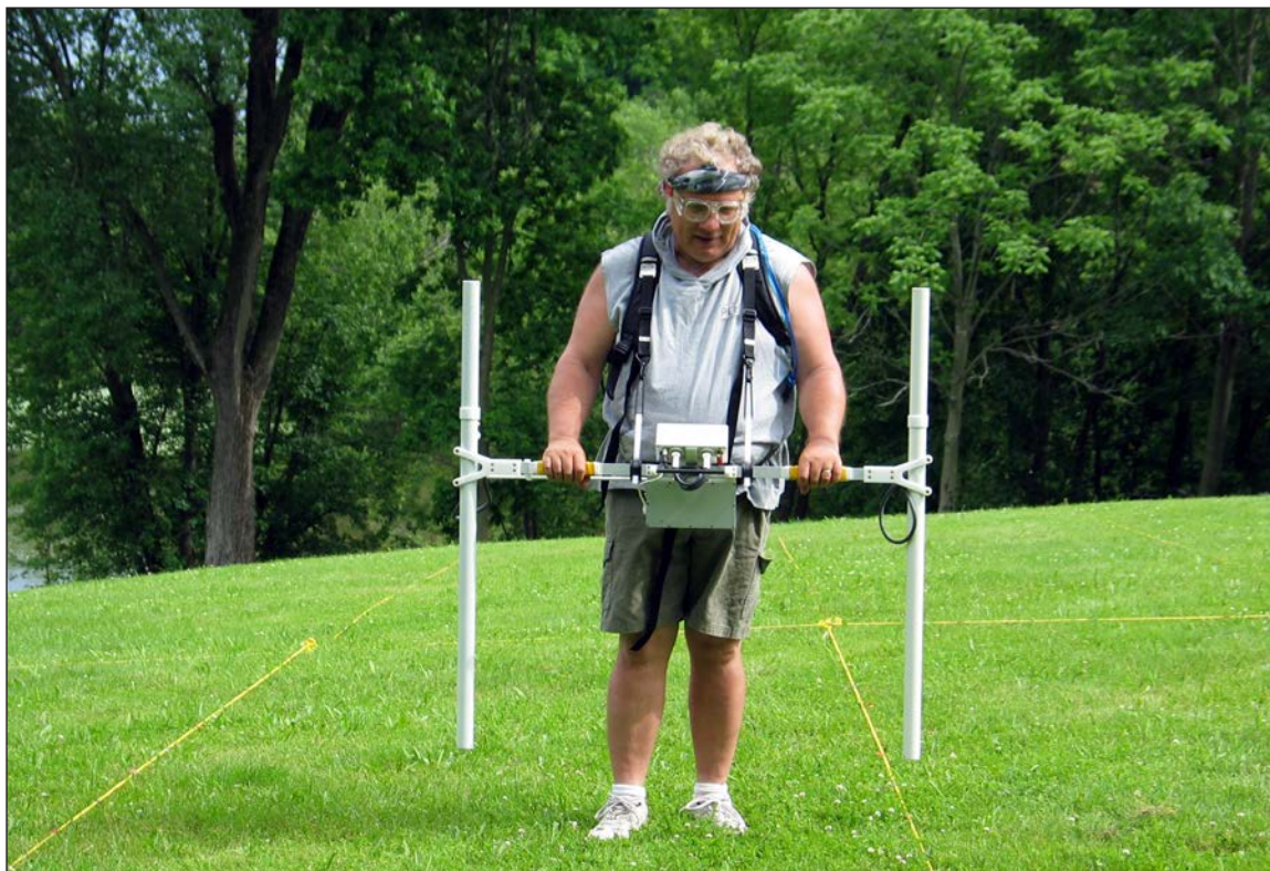
Figure 10. Conducting the magnetic survey at EFMO1 with a dual fluxgate gradiometer (view to the south).
