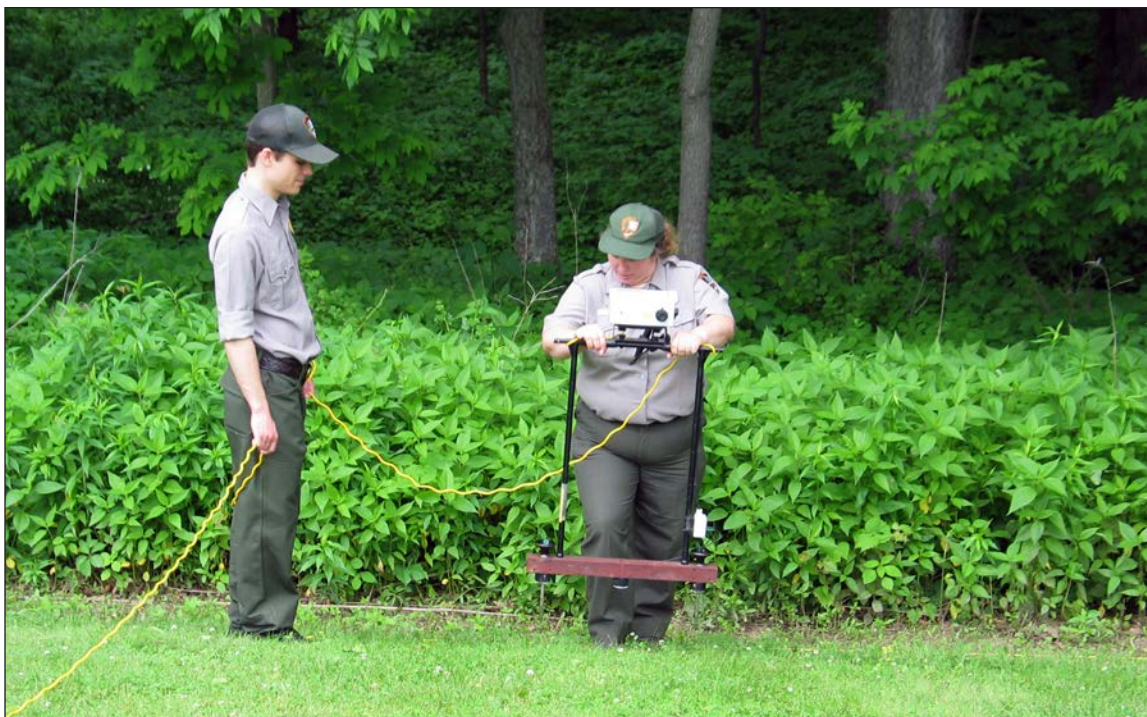
Figure 12. Conducting the resistance survey with a resistance meter and twin probe array at EFM01 (view to the north northwest).
