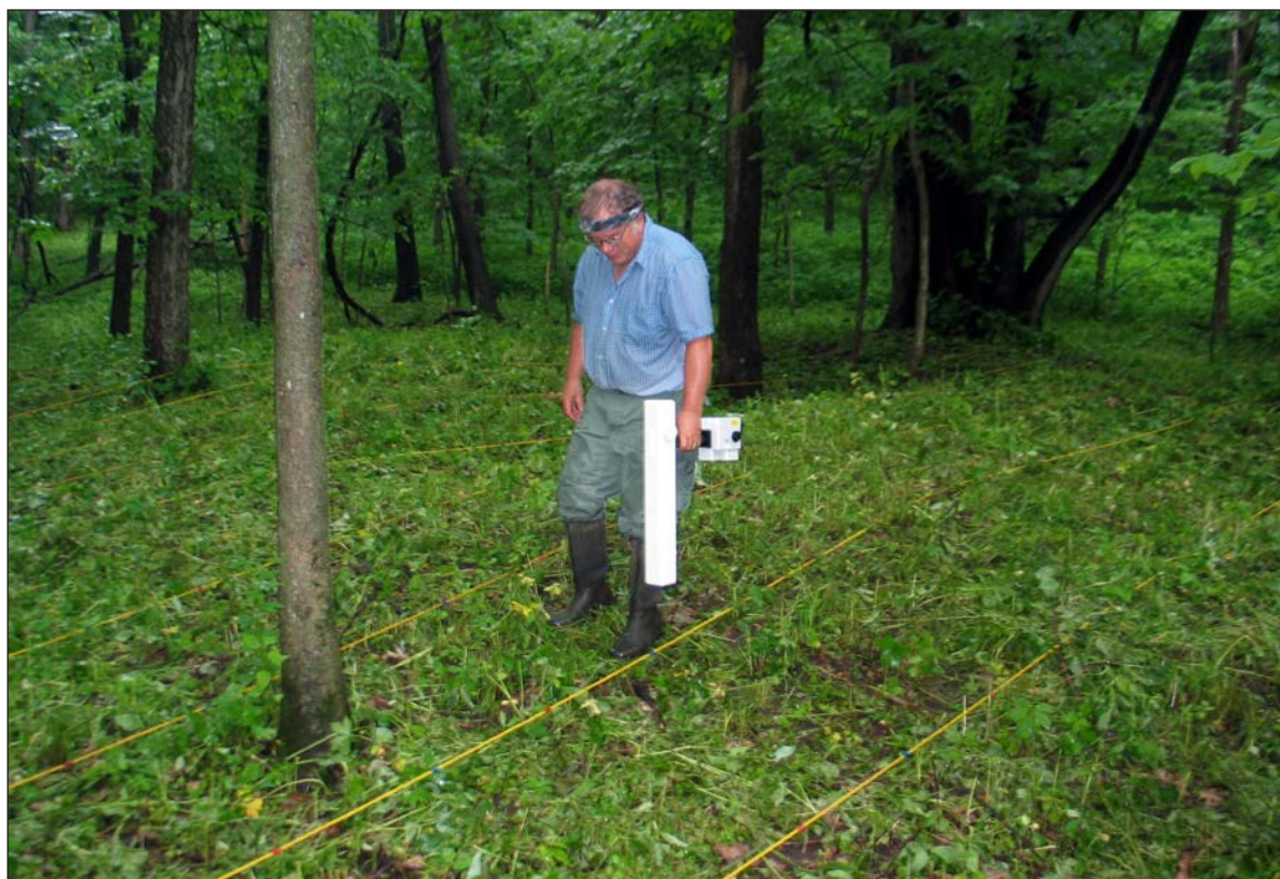
Figure 9. Conducting the magnetic survey at EFMO2 with the single fluxgate gradiometer (view to the northwest).
