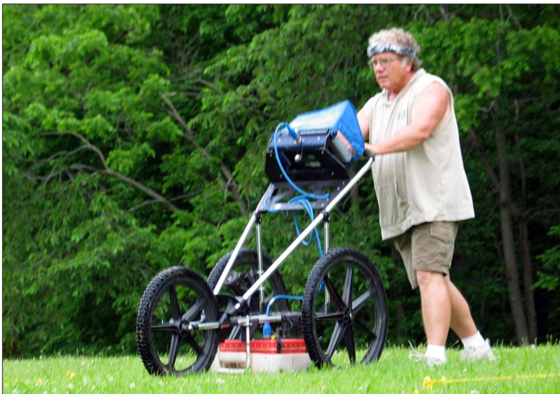
Figure 13. Conducting the ground penetrating radar survey with a gpr cart and 400 mHz antenna (view to the west northwest).
