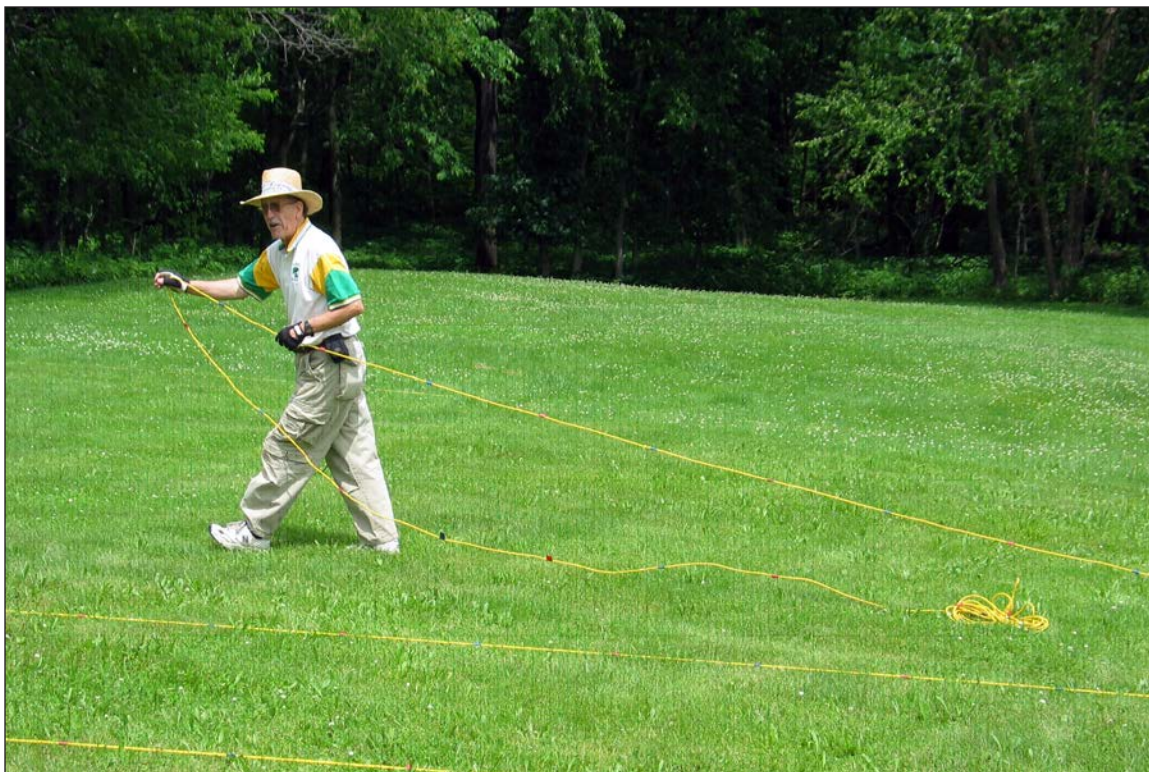
Figure 6. Laying out the survey ropes at the EFMO1 geophysical project area (view to the northeast).
