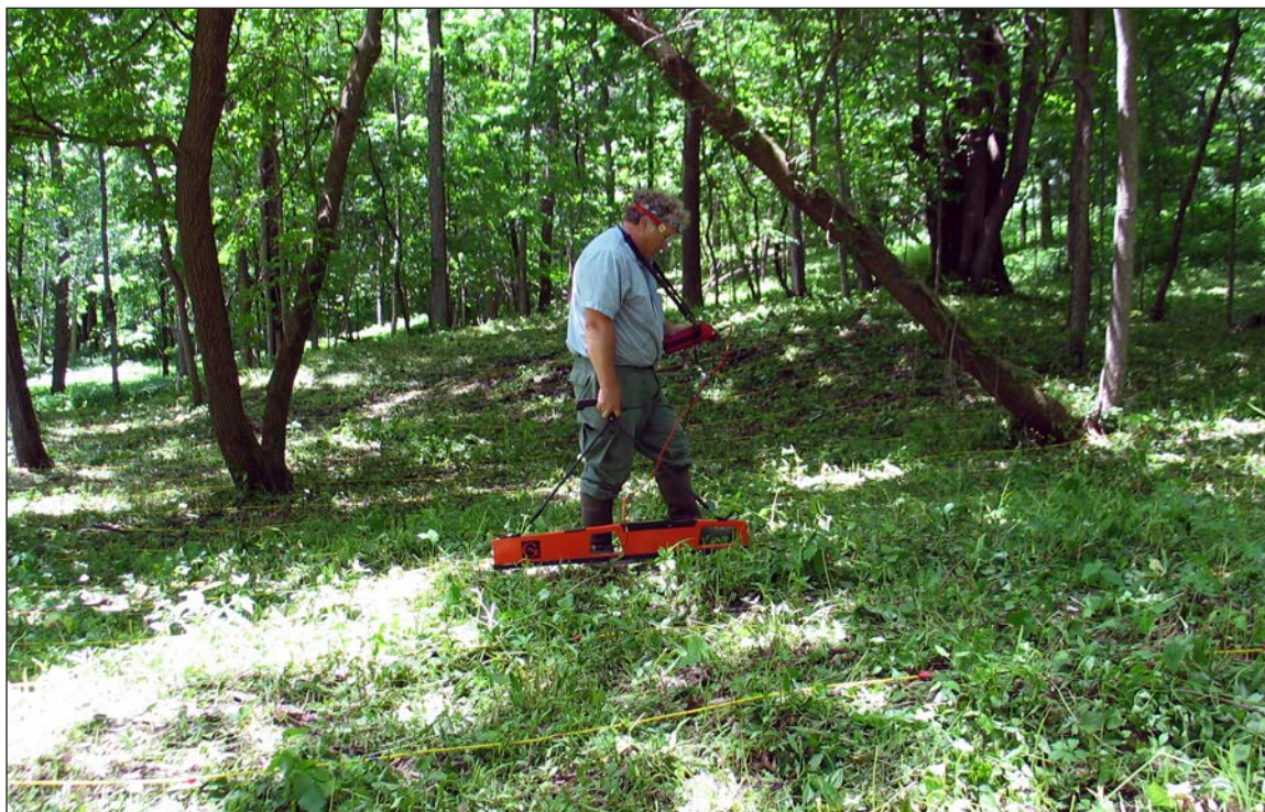
Figure 11. Conducting the conductivity survey with a ground conductivity meter at EMFO2 (view to the west).
