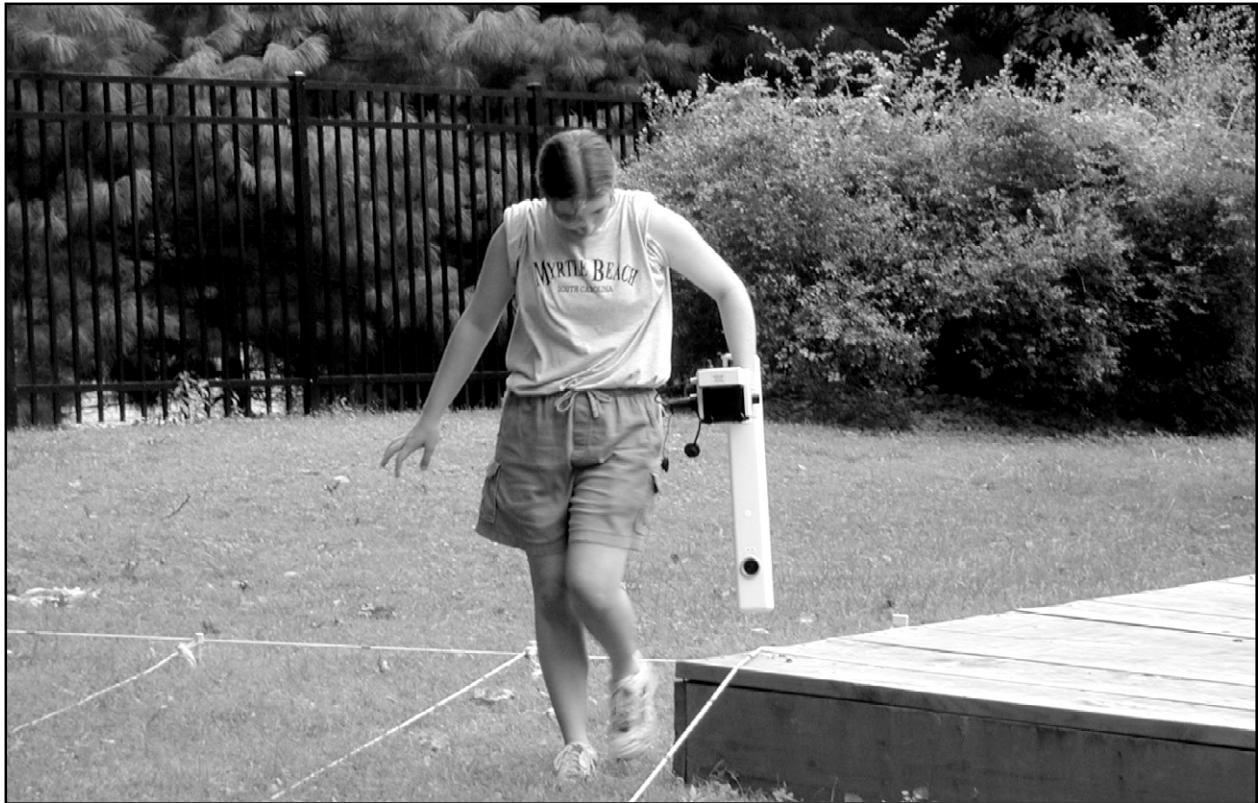
Figure 8. Anne Kern beginning a transect with the Geonics fluxgate magnetometer near the Barn Well (HS-9).
