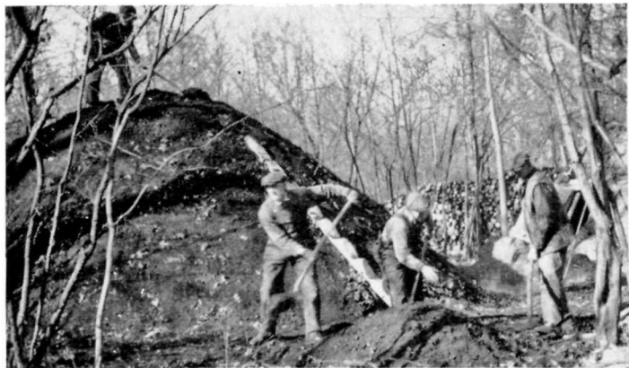
Dusting the pit
