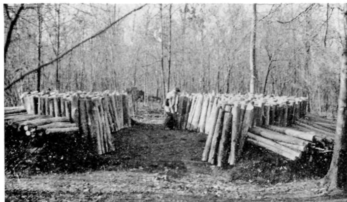
Filling a bearth with lap-wood and billets
