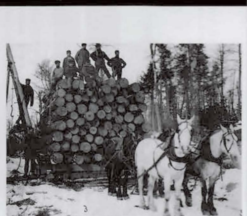
flourishing mills around the Great Lakes. (Source: State Historical Society of North Dakota) Logging was winter work as lumber crews cut the great pines and loaded them onto sleds. The trail was iced with water to enable horses to pull immense loads to staging areas along rivers for the spring log drives. Contests developed between crews to
