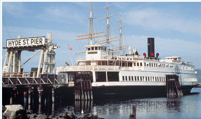
Eureka: side-wheel ferry; 299.5 feet; built in 1890 as Ukiah, Tiburon, CA; refitted 1922 as Eureka.
