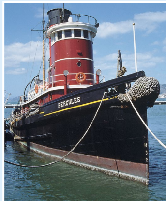
Hercules: steam-powered tugboat; 139 feet; built 1907, Camden, NJ.
