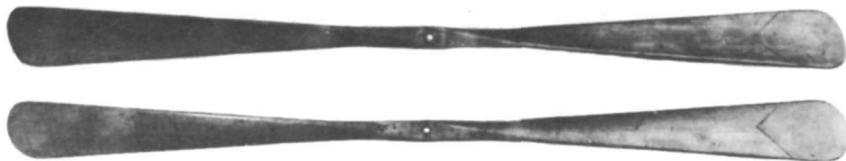
Propeller estimates, made by the Wrights 8 months before the flights of December 1903. Their formulas resulted in the highly efficient propellers which were used in the first Wright Flyer. These were 8 1/2 feet from one canvas-covered tip to the other. Top view shows the front, bottom view, the rear.
