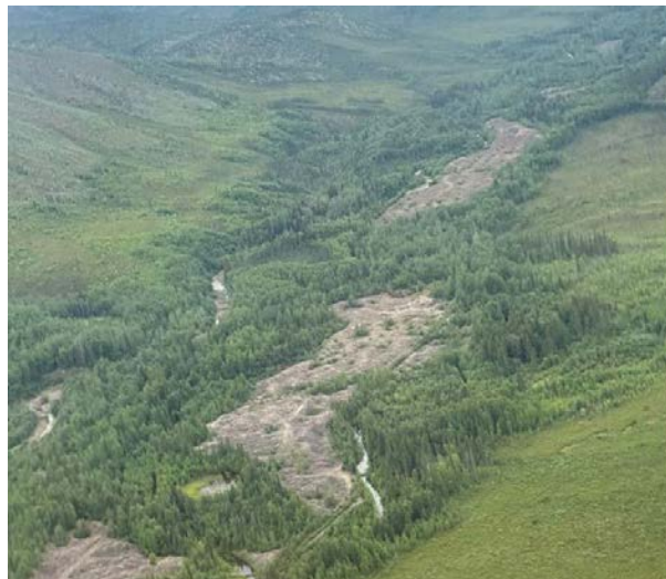
Figure 3. Aerial view of Coal Creek, in Yukon-Charley Rivers National Preserve. The photo shows the extensive mine tailings in the active corridor of the creek, which is proposed as a site of stream restoration.
