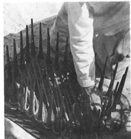
Shot line being faked onto the pin prior to shooting with lyle gun.
