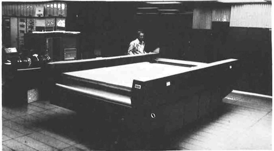
Xynetics Model 2000 Table Plotter. Computer output as land suitability data can be displayed on maps by this machine. Machine plots up to 40"/sec. using eight different colors on maps up to 6 X 10'. Photo NASA.
