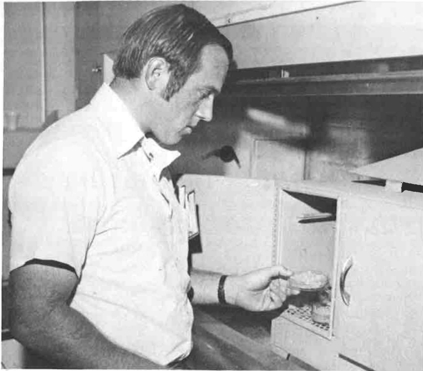
Dr. Dennis B. Fenn, research soil scientist of the Ecological Services Division, placing soil samples in a drying oven to study their drying properties.
