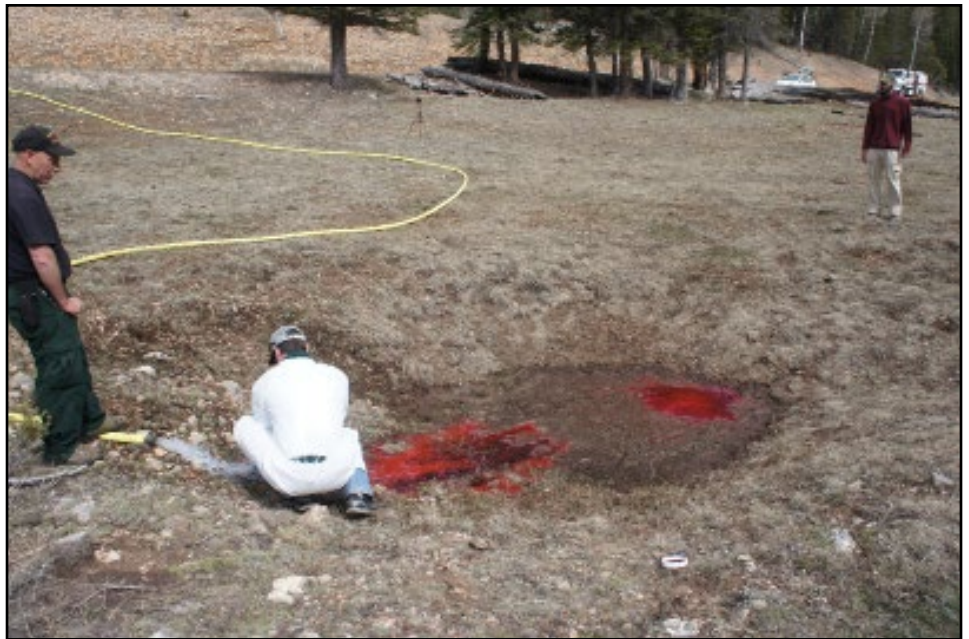
Park staff injecting Rhodamine WT into a sinkhole above the North Rim using park fire equipment to flush the dye. NPS photo.
