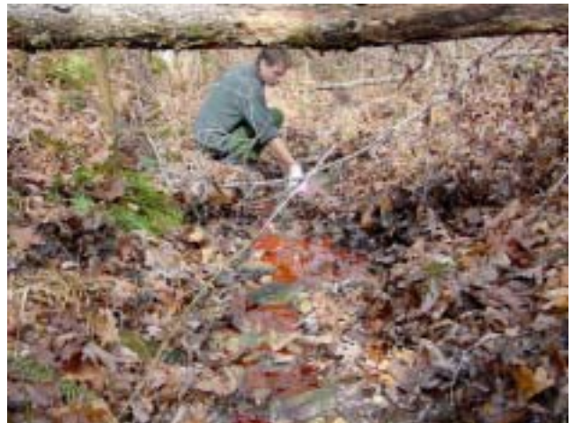
Chuck Bitting injecting rhodamine WT. (NPS photo by Noel Mays)
