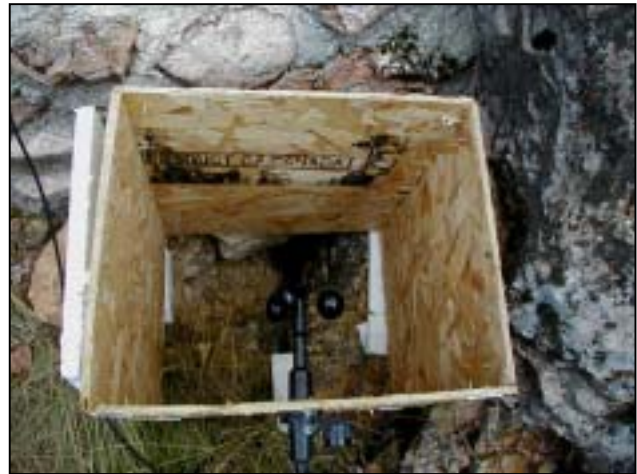
Figure 2 - The Snakepit Entrance Anemometer in the airflow enclosure. (NPS Photo)
