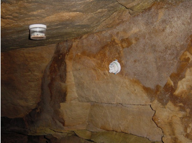
Three dataloggers were recently installed inside of fifteen Buffalo National River caves to study temperature and humidity conditions in bat roosts of endangered species.
