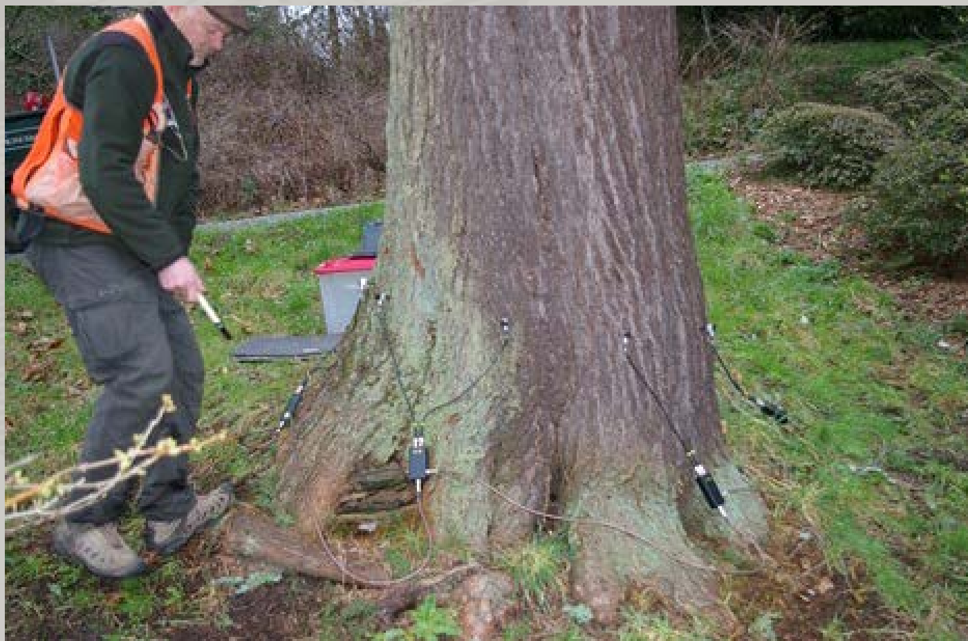
Caption: Sonic tomograph sensors attached around the base of a tree ( Univ. of WA Botanic Gardens ).
