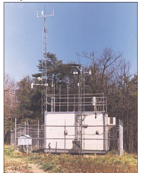
Figure 3 (below). Instruments at Look Rock record weather data, measure ozone, and analyze visibility distance (visual range). A data logger collects the information and forwards it to Sugarlands Visitor Center.
