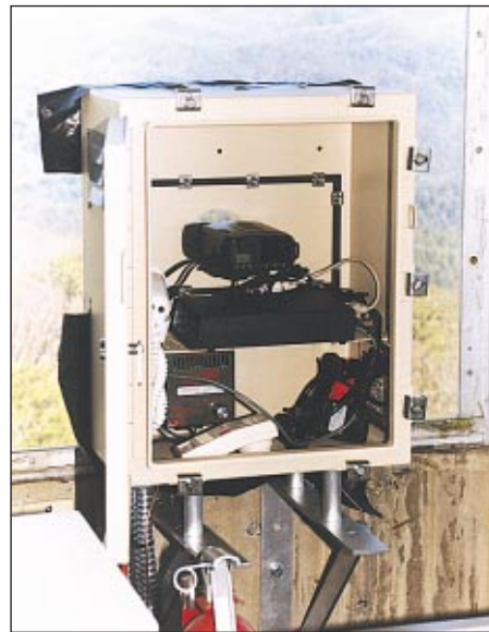
Figure 2. Capturing a new visibility image every 15 minutes, the digital camera is mounted inside the observation tower at Look Rock. The digital image is transmitted by telephone line and short-haul modem to the Look Rock air quality shelter (right).
