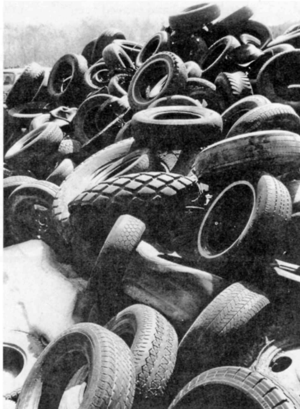
The Corps' Cold Regions Research and Engineering Laboratory (CRREL) has developed a way to recycle used tires such as these for use as road insulation. (photo courtesy CRREL)
