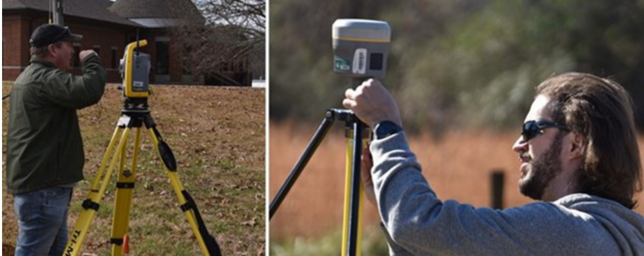
Left, Ches Vervaeke uses the surveyor's compass to collect backsight azimuth during total station setup. Right, Daniel McCay secures the connection for the RTK base station. NPS photos / Mark Hynds
