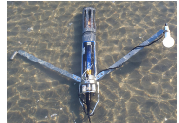
This water quality monitoring meter measures water salinity, temperature, and turbidity.
