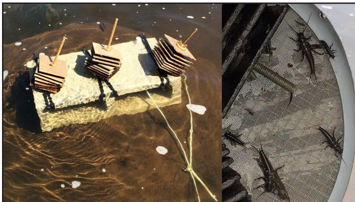
Hester-Dendy invertebrate samplers are placed at least 2 feet below the water surface where there is good streamflow. When removed, the plates are rinsed to collect aquatic insects, such as stoneflies ( right ), that have gathered on them. NPS PHOTO/R. DAMSTRA.
