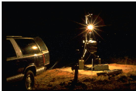
A standard UV lamp field calibration performed at night during the September '94 intercomparison.
