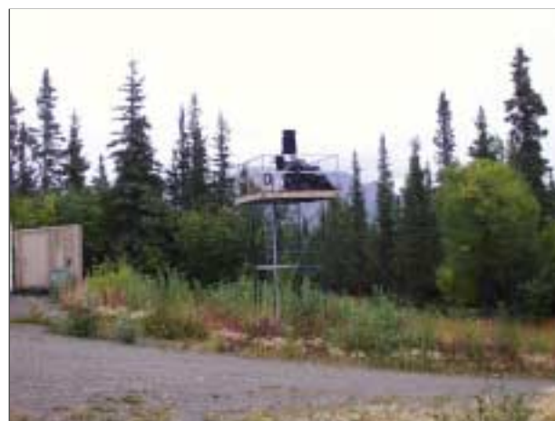
The Brewer instrument at Denali National Park is shown here with the Central UV Calibration Facility's field calibrator.
