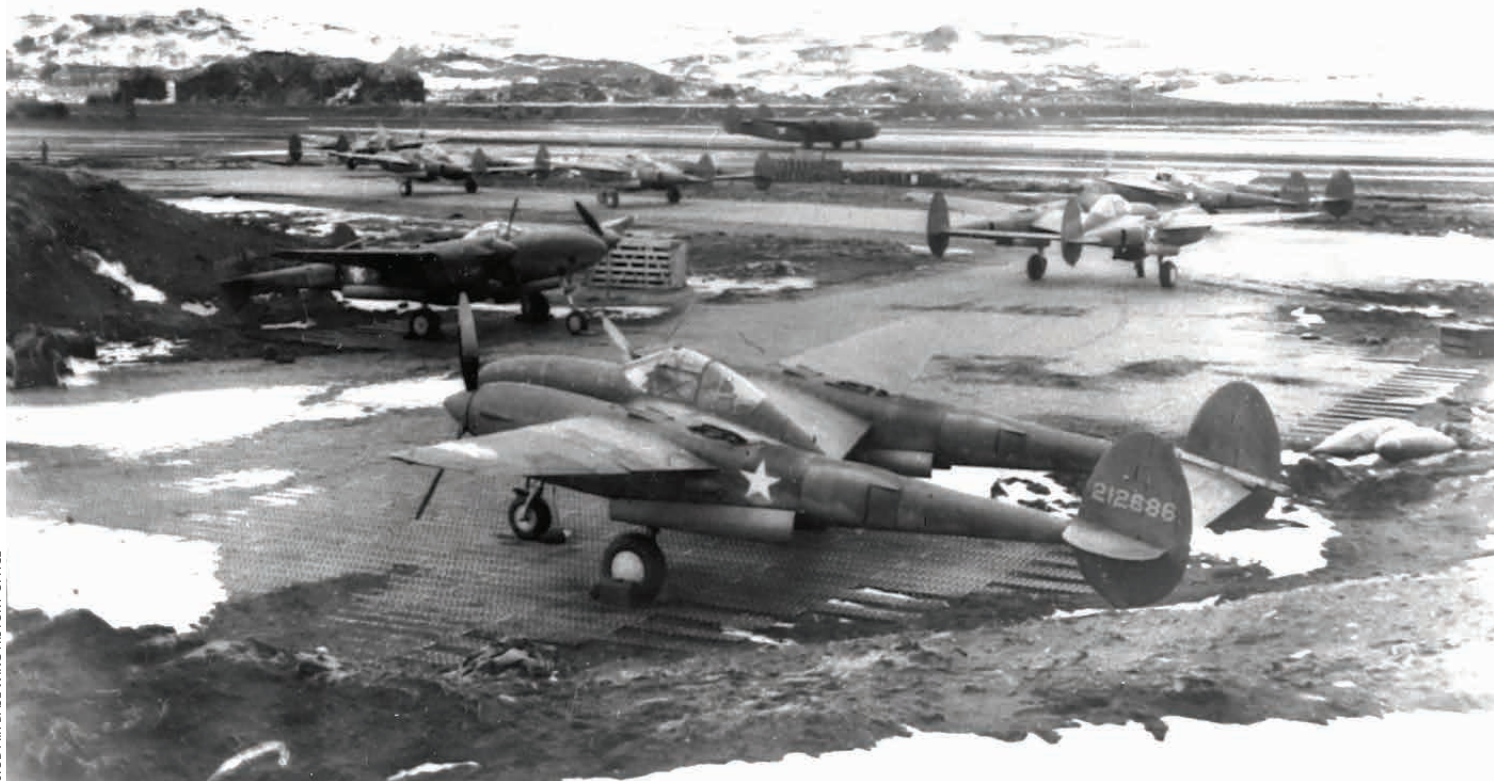
The F-5 was the “eyes” of the army. The Lightning was armed with five powerful cameras in the nose.
