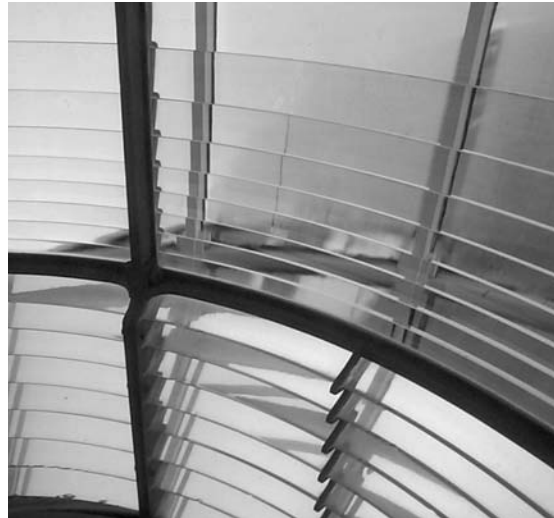
Figure 27 First order Fresnel lens.
