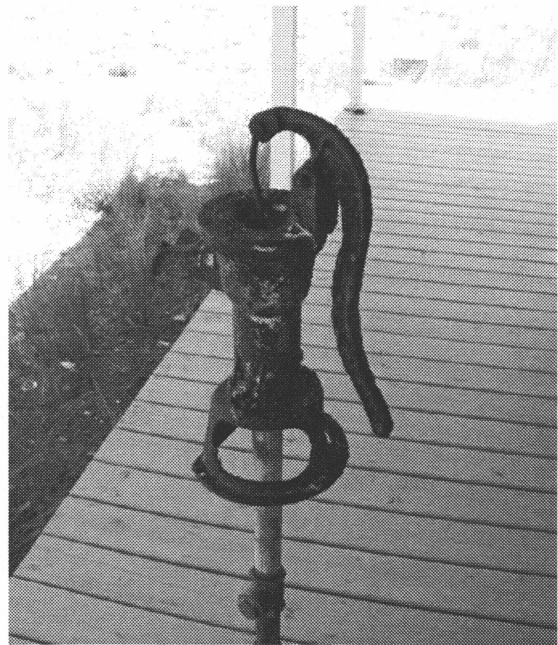
Figure 34 Hand-operated water pump on northeast porch. (NPS-SERO-CR, 2003)
