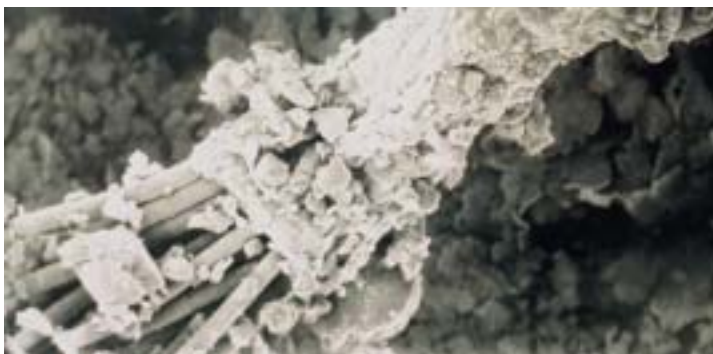
Extreme close-up: through the lens of an electron microscope (950x), the fibers holding the crust together are clearly visible.
