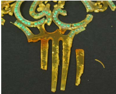
Figure 1. Severely degraded cellulose nitrate comb shows crazing, cracking, and discoloration (circled). Internal and /or surface crazing is often the first sign of degradation and precedes brittleness and fracture.
