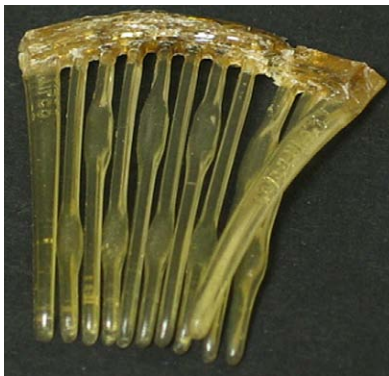
Figure 2. Distorted and discolored cellulose acetate comb; upper band has severe crazing and a white powdery bloom (circled) caused by migrating plasticizer.
