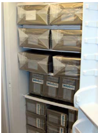
Figure 4. A freezer filled with properly packed boxes. Labels face forward for easy retrieval.
