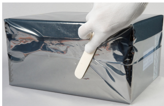
Figure 5. A bone folder is being used to “burnish” tape to ensure it adheres to the package.
