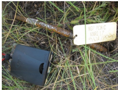
Figure 5. A sample of the center marker at an NGPN long-term vegetation monitoring plot. The rebar is bent in the field with a brass tag noting the plot number, date of installation, and location. A compass is used for scale.
