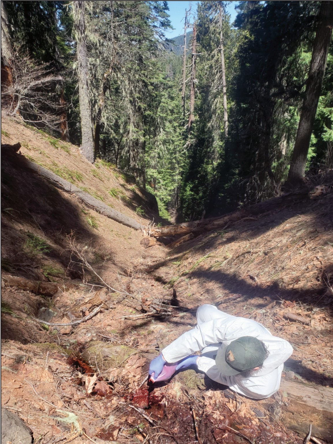
Figure 8. National Park Service employee conducting dye injection of eosine oj into a ravine in the upper Cave Creek watershed (injection I-4), April 28, 2021. The person injecting the dye is wearing gloves and a Tyvek suit to prevent cross-contamination of dye to monitoring sites or other dye injection locations. Photograph by Benjamin V. Miller, U.S. Geological Survey.
