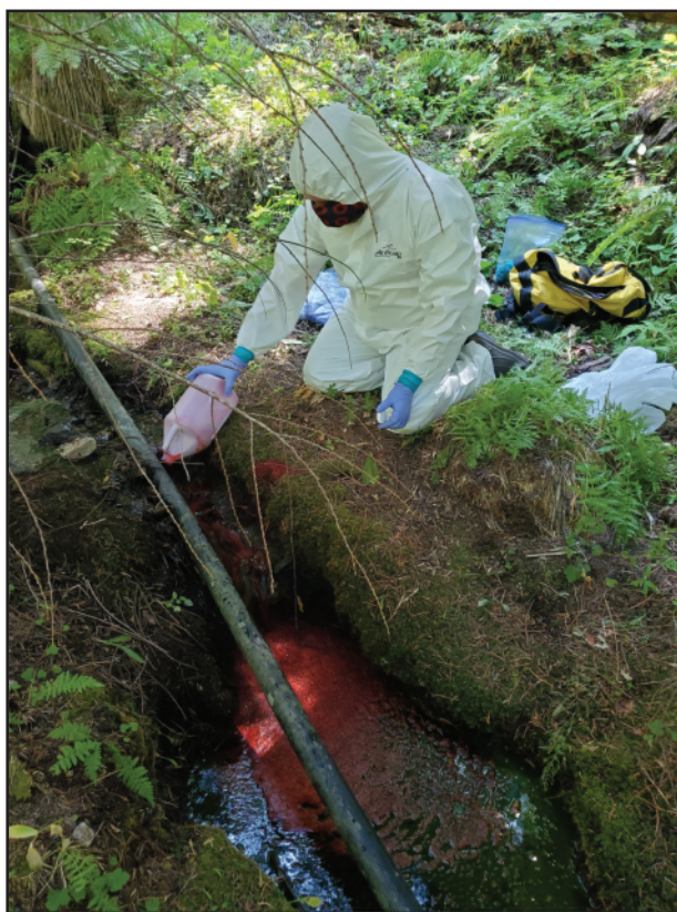
Figure 11. U.S. Geological Survey (USGS) scientist conducting dye injection of eosine oj into Panther Creek, April 26, 2021. The person injecting the dye is wearing gloves and a Tyvek suit to prevent cross-contamination of dye to monitoring sites or other dye injection locations. Employee was wearing a mask to comply with COVID-19 travel guidelines. Photograph by Benjamin V. Miller, USGS. USGS scientists followed all appropriate safety protocols and requirements for working near, on, in, or over water consistent with approved USGS Job Hazard Analysis.
