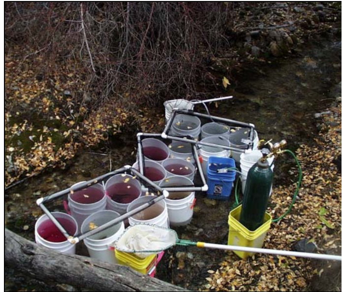
Figure 8. Toxicity test to determine amounts of antimycin and potassium permanganate needed for the treatment (2001).
