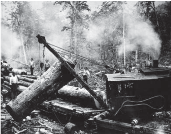
Figure 6. A log loader lifts a log onto a flatbed rail car. (NPS, "Logging," www.nps.gov/media/photo/gallery.htm?id=BF35F887-1DD8-B71C-0793D04A3C9075AF )
