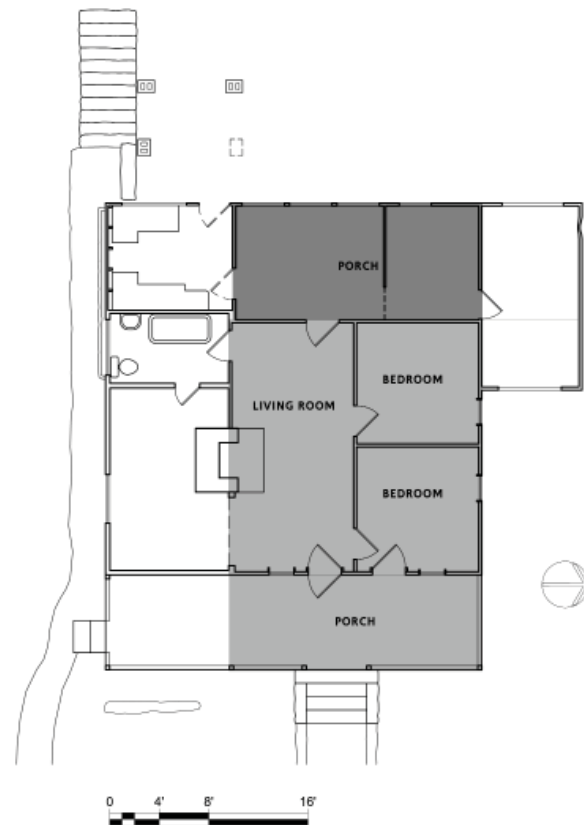
Figure 24. Floor plan showing the first phase of alterations in dark grey, the addition of a back porch the width of the building.
