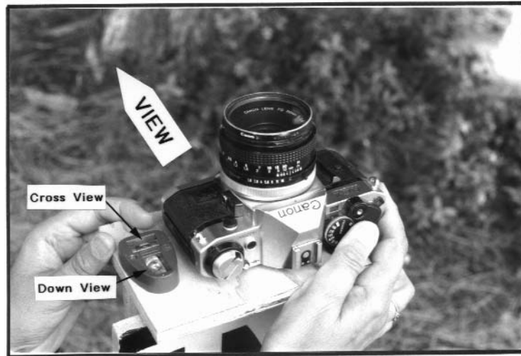
Figure 63—The camera leveling board is used to take repeat photographs of the tree canopy with some consistency. Place the leveling board on top of the meter board for consistent height above the ground. Place the meter board at right angles to the photo view. Move the meter board sideways to center the cross-view bubble, then tilt the level board to center the down-view bubble, move your head back, and photograph.
