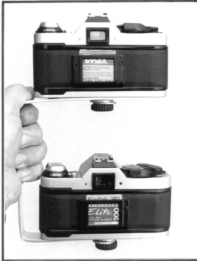
Figure 64—Double camera bracket for use when photographing in both color and black and white. The bracket is made from 1-inch by 1/8-inch aluminum bar-stock with holes drilled to mount the cameras. Identical cameras are recommended to simplify camera adjustments. Figures 65 and 66 illustrate construction details.
