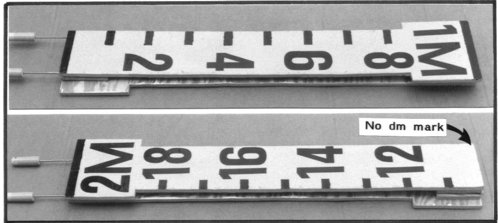
Figure 54—The 2-meter board system. In the top photo, a standard 1-meter board is shown with the 2-meter half folded under it. In the bottom photo, the folded board has been turned over showing the 2-meter section. “No dm mark” designates the lack of a decimeter mark at the base of the top board; it is at the top of the 1-meter board shown directly above. Length of the 2-meter section must be 2 centimeters shorter (exactly 1 meter instead of 1 meter 2 centimeters) than the 1-meter board to account for this decimeter mark.
