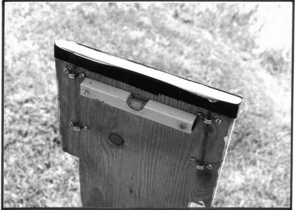
Figure 52—A line level is used to orient the board vertically. Obtain a 4- to 5-inch-long (10- to 12-cm) line level and drill a hole in each end for a screw. Attach one end of the line level to the back of the meter board \frac{1}{2} inch (1 cm) from the top. Then orient the board vertically by using a carpenter's level along one side. Hold the board in position, adjust the line level to horizontal, and carefully screw in the other end.
