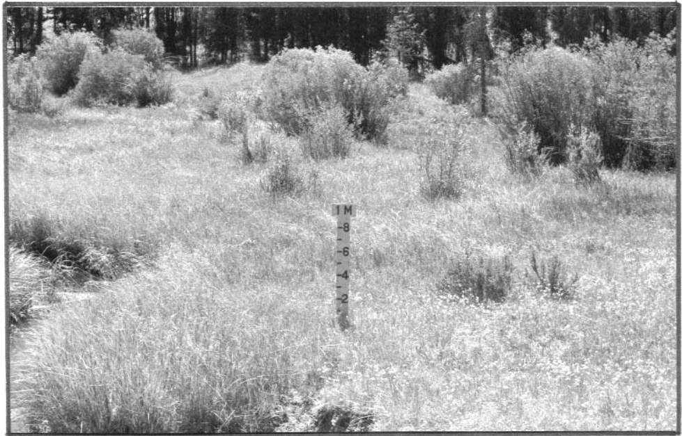
Figure 35—A 1981 view of the Pole Camp wet meadow photo point, which will be used to illustrate grid analysis. This photograph will be compared to one from 1996. The first step is to attach a clear plastic outline form (shown in fig. 36). Fill in the required site information and outline the shrubs (fig. 37).
