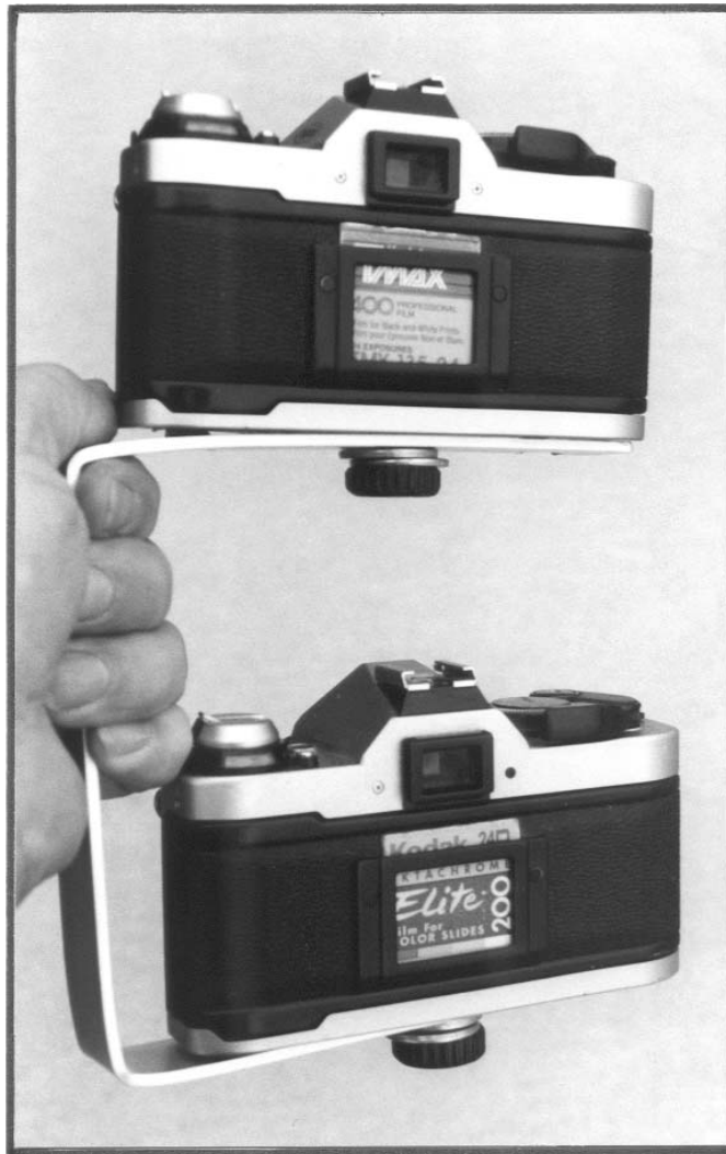
Figure 29—A system for combining color and black-and-white photography. Both cameras are connected by strap aluminum 1/8 inch thick and 1 inch wide bent into a “U” with holes drilled for mounting screws to connect the cameras (see app. B for details). The cameras operate independently. Identical cameras simplify the photography because all control settings are adjusted in the same way, which helps in avoiding mistakes. Shown here are cameras with black-and-white film at 400 ISO and color film at 200 ISO.
