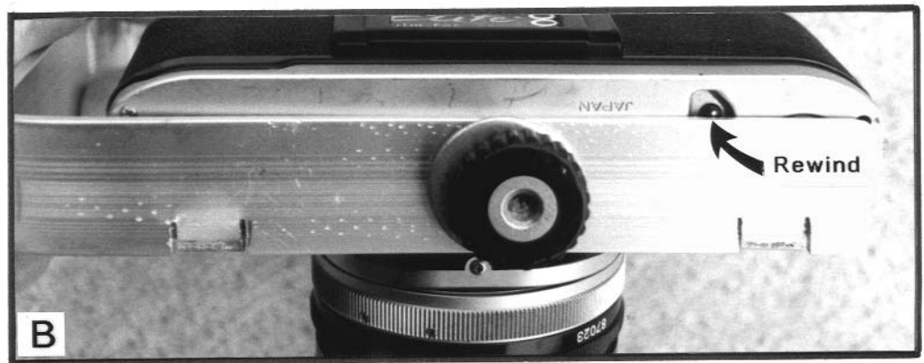
Figure 66—Two factors are important in attaching a camera to the bracket. (A), Make two cuts \frac{1}{4} of an inch deep and \frac{1}{2} inch apart into the front of the bracket. Bend up to about a 30-degree angle to prevent rotation movement of the camera. (B) Make sure the bracket clears the rewind button so that film may be changed while the camera is attached to the bracket.
