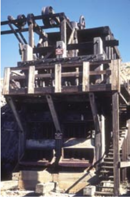
The Lost Horse Mill site, listed on the National Register, is the only ten-stamp mill within the park.
