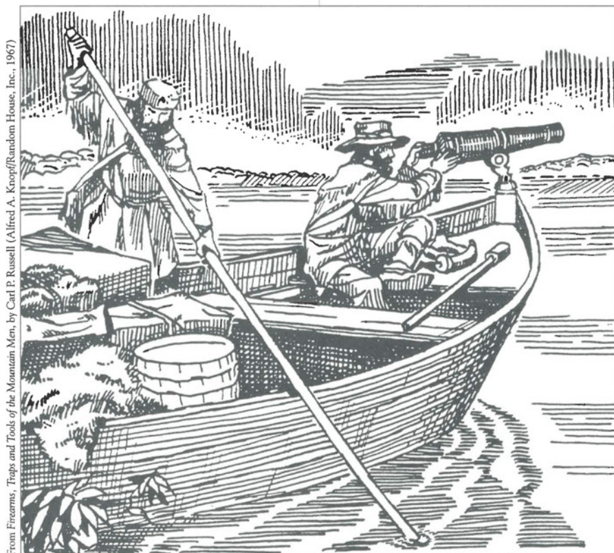
Figure 7. The expedition carried a swivel-mounted cannon on the keelboat, the largest piece of ordnance on the Missouri River. Smoothbore, it could fire either a large solid shot or a group of musket balls.
