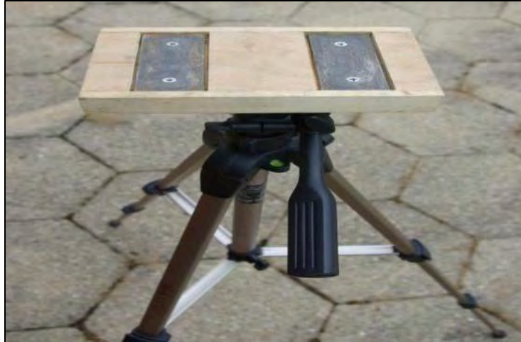
Figure SOP2-7. Tripod “pan-head” with laser assembly mounting frame. The frame is attached to the tripod’s quick release mounting plate, showing the 2 laser seats with steel floor-plates for magnetic attachment of laser units. Note tripod leveling bubble to the left of the “pan-head” handle.
