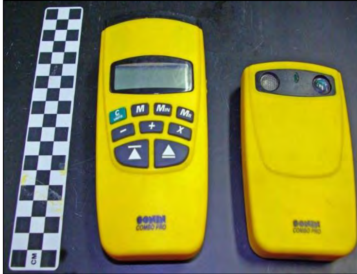
Figure SOP3a-8. The Sonin Combo Pro™ electronic rangefinder includes a transmitter (left) and a receiver (right).
