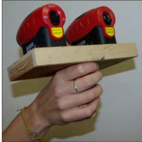
Figure SOP2-8. Handheld strip generator. This is used to determine cave cricket cluster size by measuring distances among neighboring cave crickets in a cluster.
