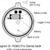
Diagram B- HOBO Pro Series back with cover removed
