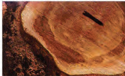
Figure 1. One to two inch-wide, crescent-shaped bands of stained and/or decayed wood in the inner outer heartwood.
