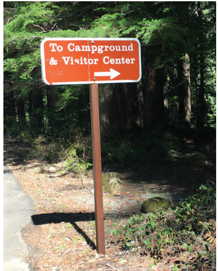
Figure 81. Aluminum wayfinding sign, 2017. This style of wayfinding sign is suitable for signs intended to be seen from moving vehicles. Source: NPS.
