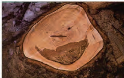
Figure 5. Decayed wood surrounded by stain. Decay is laminated, separating at the annual rings.
