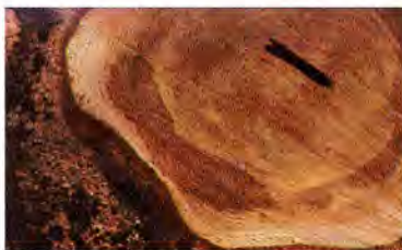
Figure 1. One to two inch-wide, crescent-shaped bands of stained and/or decayed wood in the inner/outer heartwood.
