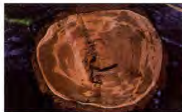
Figure 2. Stain and decay in the inner heartwood and the sapwood.
