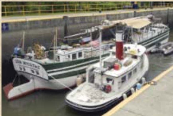
The Lois McClure transformed into a traditional canal boat with mast and sails lowered to accommodate the Erie Canal's famous low bridges. Her trusty tug, the Churchill—the modern equivalent of mules or horses that towed canal boats in the 1800s—pulled her from port to port.
